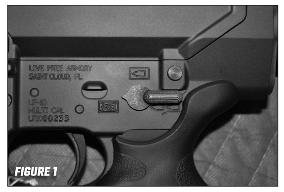
WARNING: THE FIREARM SHOULD ALWAYS BE PLACED ON "SAFE" EXCEPT WHEN FIRING. ALWAYS VISUALLY CHECK THAT THE SAFETY IS IN ITS INTENDED POSITION.
